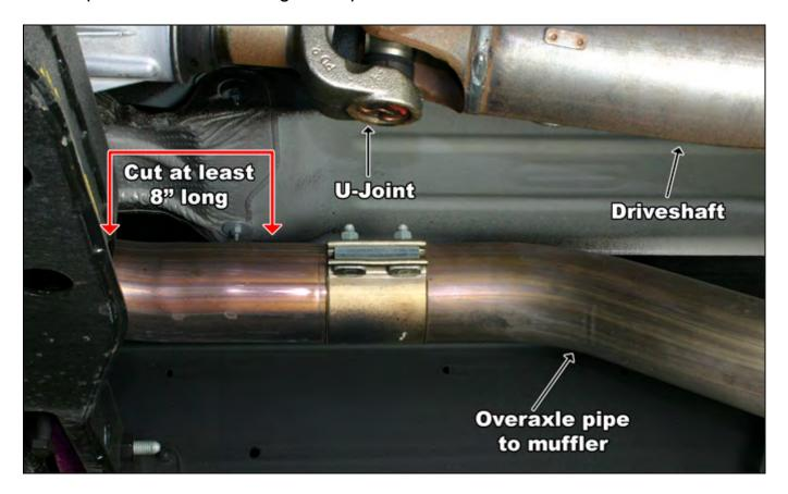
Remove the 8" section of pipe with a sawsall or cutoff saw.
