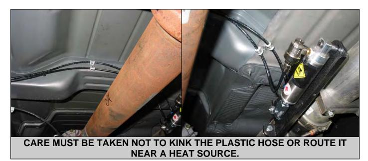
Insert one end of the remaining ¼" hose into the straight fitting of the solenoid valve and route this hose as well as the plastic hose with the yellow snorkel filter along the frame rail and into the engine compartment. The hose from the solenoid valve will later be attached to the regulator on the air compressor assembly when that is installed. The hose with the filter can be run through the firewall and secured under the dash area, away from any moving or heated equipment.
