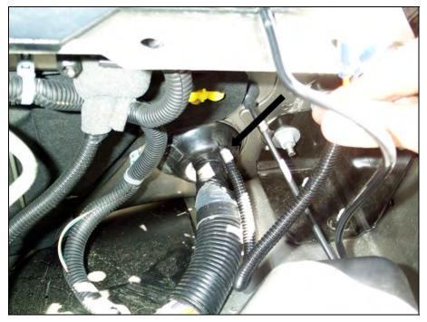
Push the black wire with the male bullet connector through the firewall grommet and connect it to the female bullet connector on the black wire coming from the brake controller module.
