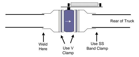
Once you have finalized the fit by welding the front flange and securing the rear the flange, tighten the two supplied V-band clamps around both flanges on either side of the exhaust brake. The exhaust brake should now be held securely in place.
