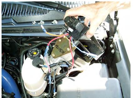
Position the air compressor assembly under the firewall flange into the cavity under the corner brace. Adjust the mount plate so that the upper 2 brace mounting bolts pass through the holes in the plate.
