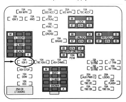
located in the diagram to the left) then install the brass fuse tap provided onto the HOT side of fuse which will be the side with power to it when the fuse is removed and key on.
