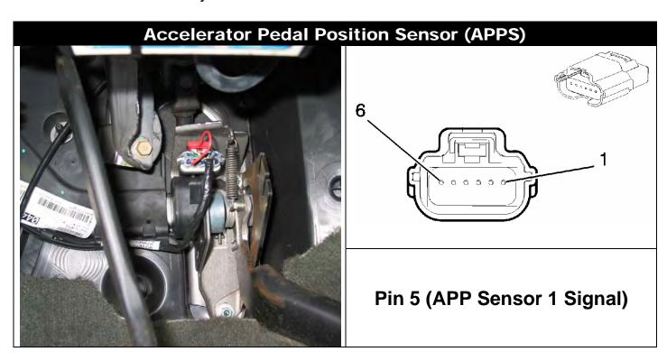
At the throttle pedal, locate the **accelerator position pedal sensor** (APPS) plug and find the **dark blue** wire located at **pin 5**. Use the provided gray (or red) Posi-Tap connector to tap onto this wire. This wire should be routed to the TPS/APPS input of the brake controller module.
