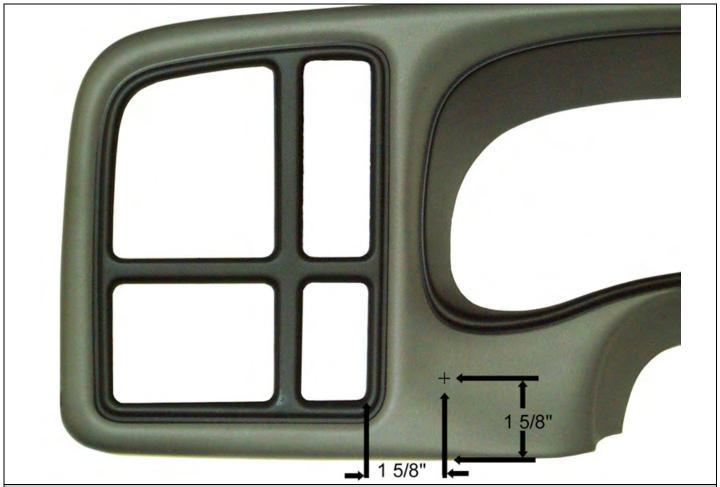
Note: This measurement must be exact as possible to ensure room for the switch on the inside of the panel.
