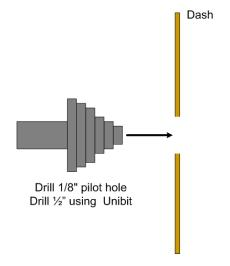
6. Once you have the mounting hole drilled, crimp the switch connectors to the switch wires and install the correct switch wires to the correct switch terminals, then insert the switch into the dash from the backside.
