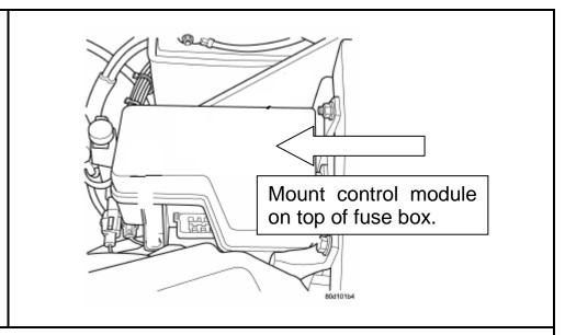
13. Double check all wiring connections and ensure wires are routed away from any heat sources and moving parts.
