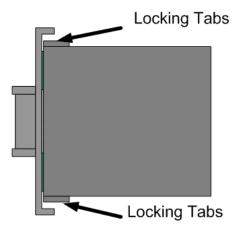
6. Change the position selection switch to position #2 (Auto Test). Slide enclosure cover over circuit board.
