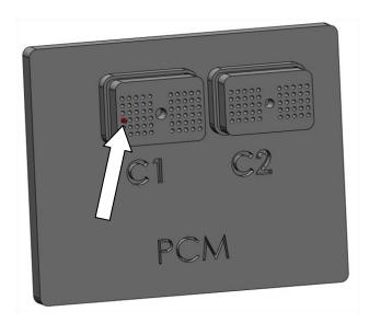
9. Being that the RPM signal is critical you will need to solder the connection.
