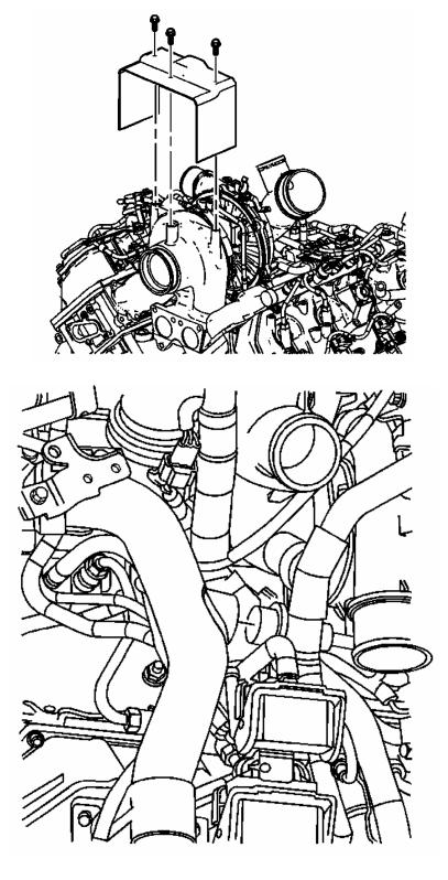
Reposition the hose clamp and remove the turbocharger outlet coolant hose from the turbocharger.
