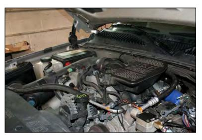
Using a 1/2" breaker bar, relax the belt tensioner and remove the belt.
