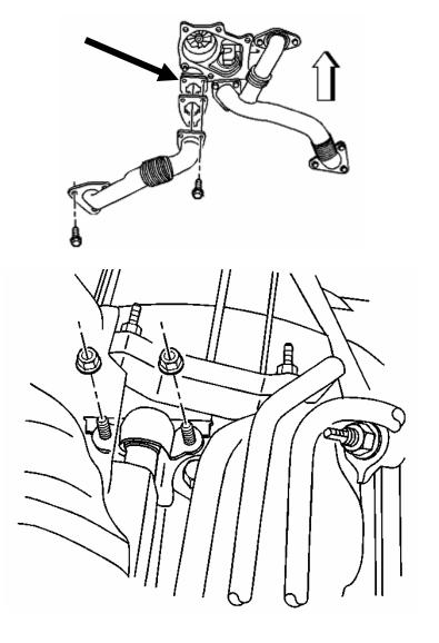
Remove the turbocharger oil feed pipe banjo bolt and washer.
