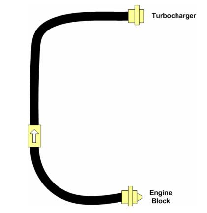
Thread the upper oil line into the exit/output of the check valve. Thread the lower oil line into the entry/input of the oil line. Both these threads are pipe threads, so do not use Teflon tape. A very small amount of liquid pipe dope may be used.
