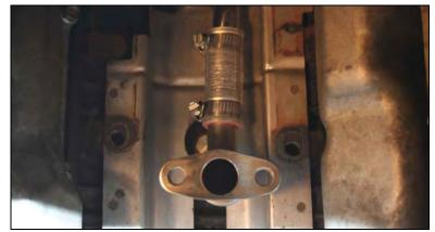
Install the two step studs for the oil drain spacer into the bottom of the turbo and tighten with double nuts. Install the oil drain spacer with a gasket on each side.
