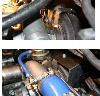
Install the stock air intake plenum to the turbo using the stock air intake V band clamp.
