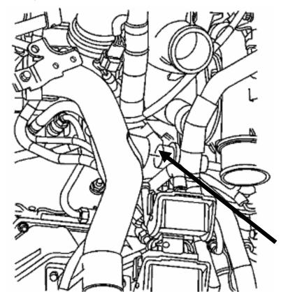
You will need to cut the oil drain tube. Cut the tube in about the middle of the straight section. Thereby ensuring that there is enough room on either side of the tube to slide the silicone adapter in place.
