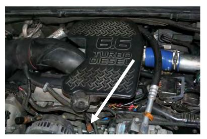
You can use an extra piece of reflective heat shielding to protect the A/C line that runs over top of the turbo. Re-install the belt and refill the cooling system. Re-install the intake silencer plenum.
