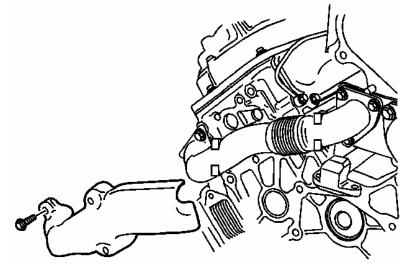
Using a 12mm - **12 point** socket, remove the six upper feed pipe bolts. Note that they may extremely difficult to remove and may require heat to break them loose or penetrating oil.
