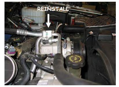
Using a 1/2" breaker bar, relax the belt tensioner and reinstall the belt.
