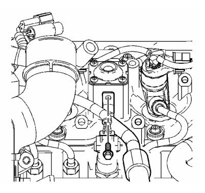
Remove the left PCV hose/pipe bolt.
