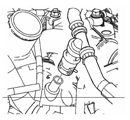
Reposition the positive crankcase ventilation (PCV) hose clamp.
