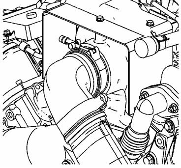
Loosen exhaust outlet clamp and remove exhaust down pipe.
