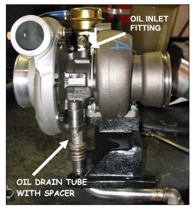
Install the oil drain gasket on the two studs on the block. Pay attention to the proper orientation of the gasket. Remove the old gasket residue first before applying the new gasket.
