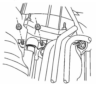
IF YOU HAVE BD'S NEW HIGH FLOW DURAMAX MANIFOLD, YOU SHOULD INSTALL IT NOW. AT THIS POINT MAKE SURE THAT ALL BOLTS HAVE BEEN TIGHTENED, ALL BOLTS THAT WERE SNUGGED UP WERE TO AID IN FITMENT ADJUSTABILITY.
