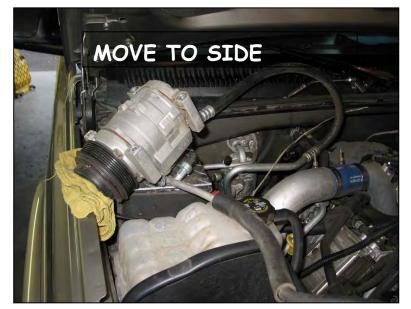
Using a 7/16" deep socket, remove the compressor outlet clamps and remove the silicon boot. The charge air cooler piping can then be pushed down towards the valve cover, and out of the way.
