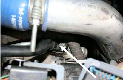
Using a 15mm socket, reinstall the four A/C compressor mounting bolts.
