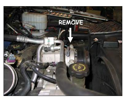
Using a 15mm socket, remove the four A/C compressor mounting bolts to move the A/C compressor for easy access to the turbo assembly. Be careful not to discharge the A/C line.
