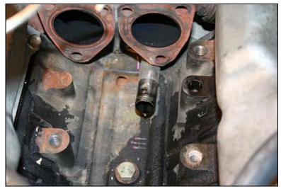
Install the drain tube with extension in place so as to line up with the turbo.
