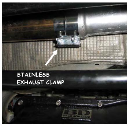
Install the new BD Turbo heat shield with two flange head bolts removed from the stock heat shield.
