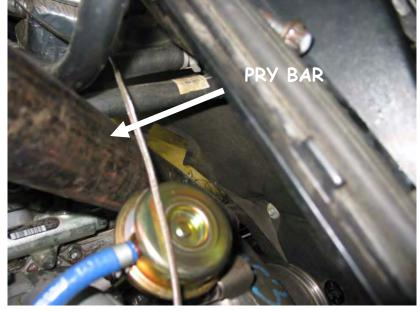
PLEASE NOTE THAT IT IS CRITICAL THAT SUFFICIENT ROOM IS MADE AVAILABLE FOR THE EXHAUST DOWN PIPE. FAILURE TO DO SO WILL CAUSE THE EXHAUST PIPES TO VIBRATE AGAINST THE FIREWALL.
