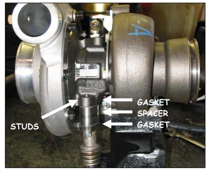
There are three paper oil drain gaskets: two are the same for the upper spacer adapter and one that is different for the tube to engine block connection.
