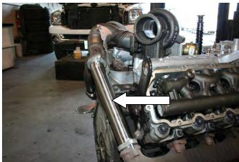
Re-install the newly supplied passenger side feed pipe using the existing hardware. Install the supplied gasket (#1900004) on the top side of the pipe. Tighten the two 10mm bolts to 30 ft lbs.
