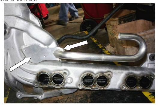
Install newly supplied (#1900003) O-ring on the EGR Cooler Bypass Pipe then install pipe into the bottom of the intake. Install newly supplied gasket **(#1900005)** and the blocker plate over the exhaust port and tighten to 100 inch lbs of torque. (NOTE: This plate secures the new pipe in place).
