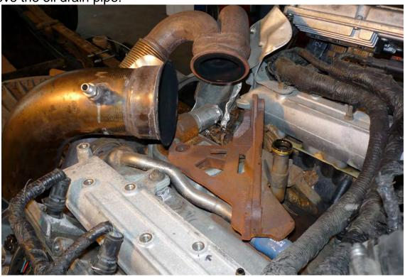
Remove the FICM (Fuel Injection Control Module) by removing two (2) 10mm mounting nuts and two (2) 8mm bolts. Disconnect the three (3) electrical plugs from the wiring harness.
