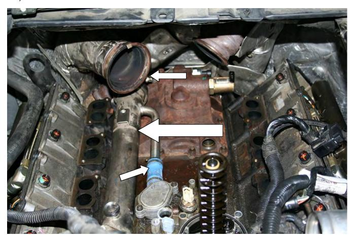
Remove the EGR cooler by disconnecting the clamp at the exhaust feed pipe then remove the coolant hose by first cutting the front clamp then twisting to align the release tab and pulling (you may have to spread the tab with a small pick or screwdriver).
