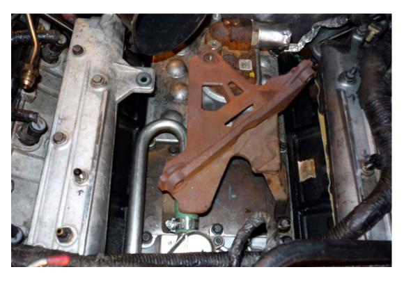
Install turbo oil drain with new O-rings.
