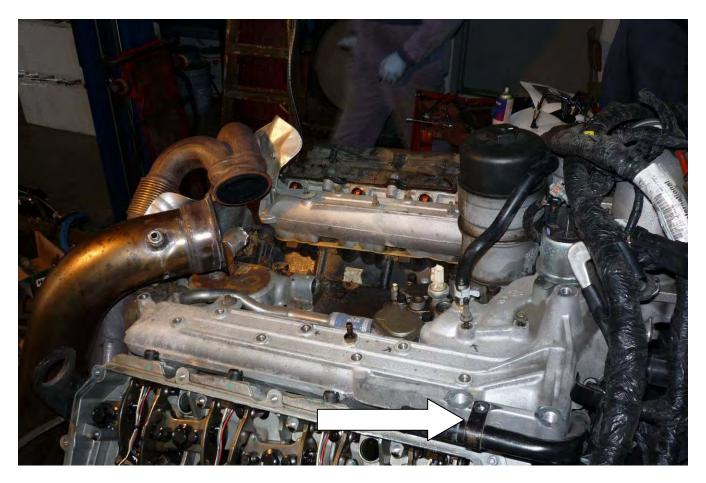
NOTE: Bend back the tab on the rigid metal tube at the RH side of intake manifold to allow manifold to clear.
