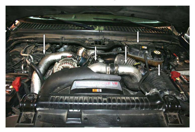
Remove the air cleaner assembly by disconnecting the MAF sensor and Filter Mind device. Then remove the ribbed hose, then the air box. Remove the two (2) 8mm bolts securing the hard tube. Then remove the breather tube from the vent on the driver side rocker cover. (NOTE: Wiggling and pulling out on the tube will help in removal).
