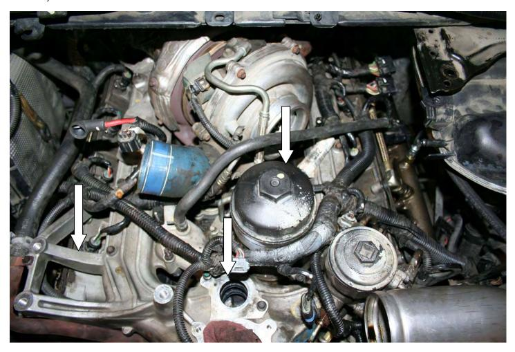
Remove the oil filter and EGR valve and service both as required.
