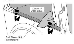
Wrap the straps on the front of the Duster™ Deck Cover around the sport bar and the bows. Thread the end through the buckle.
