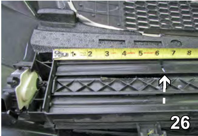
26. On the backside of the fascia, locate the top louver of the air shutter system, measure and mark over 6-1/2" from the left end of the air shutter system. Using the diagonal cutters, make a vertical cut across the louver and remove the 6-1/2" end portion. Do this to both sides of the vehicle. Driver side is shown.
