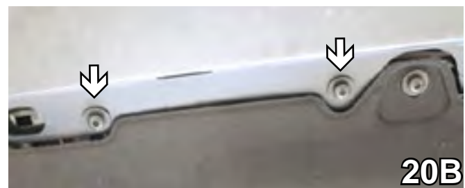
20. Optional: To install a breakaway switch, you must remove the belly pan with a T30 Torx. Remove four bolts (total) from in front of both the driver's and passenger's side tires and follow the pan toward the middle of the vehicle removing the three specified bolts (A and B). Total of seven bolts. Set all bolts and pan aside to be reinstalled later.
