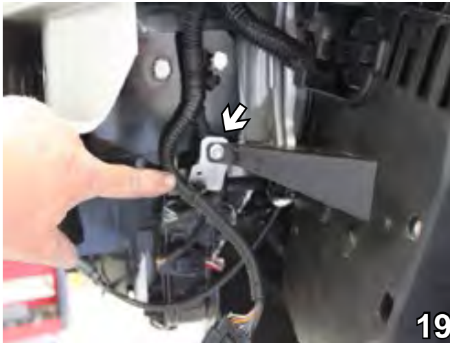
19. Bend the webbing bracket back to its original position and reinstall the 10MM bolt.
