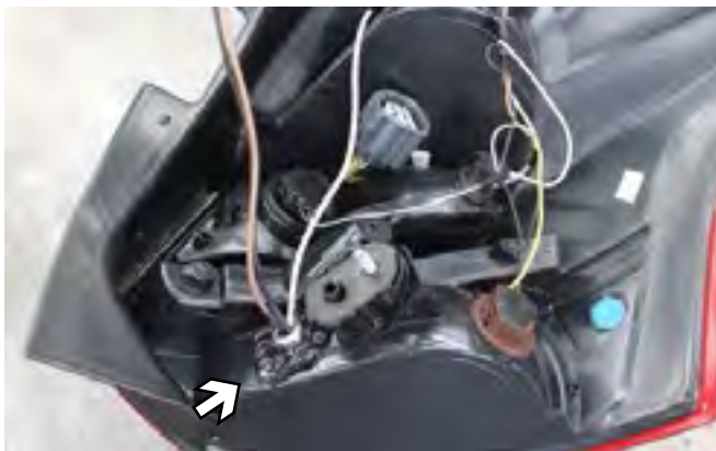
Possible location for the Bulb and Socket Wiring Kit (BX8869).
