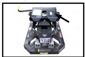
6. Verify that all fasteners have been tightened securely and the BedSaver™ is level.
