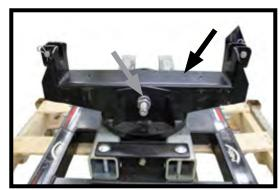
2. Using a 3/4" socket, loosen the 3/4"-10 nut (grey arrow). Remove the 3/4"-10 bolt and nut. Take the rocker arm (black arrow) off and place on a flat, steady surface.
