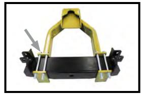
4. Insert the four (4) 1/2"-13 x 5-1/2" hex head bolts, 1/2" lock washers and 1/2"-13 hex nuts. Tighten securely.
