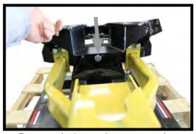
5. Re-attach the rocker arm and BedSaver<sup>™</sup> assembly to the hitch base using the 3/4"-10 bolt and nut that was previously removed. Tighten securely.
