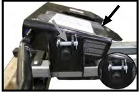
1. Remove the two (2) rocker arm clevis pins, one (1) per side (grey arrow). Remove the plate assembly from the hitch base (black arrow).
