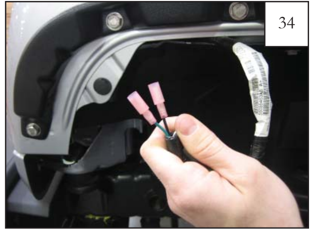
Install a Female Bullet Connector to the end of each factory side marker light wire and secure by pressing firmly with a wire crimp.
