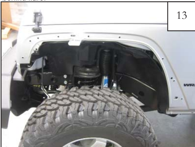
Hold splash shield up to inner wheel well to ensure that the edge is flush with the sheet metal. Remove from wheel well and trim or sand if splash shield extends beyond the sheet metal.
