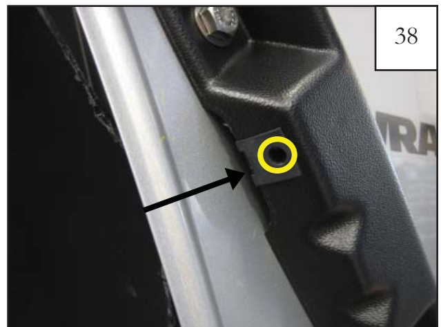
Before installing the outer flare, make sure that the speed clips on the inner pieces are centered over the predrilled holes.
