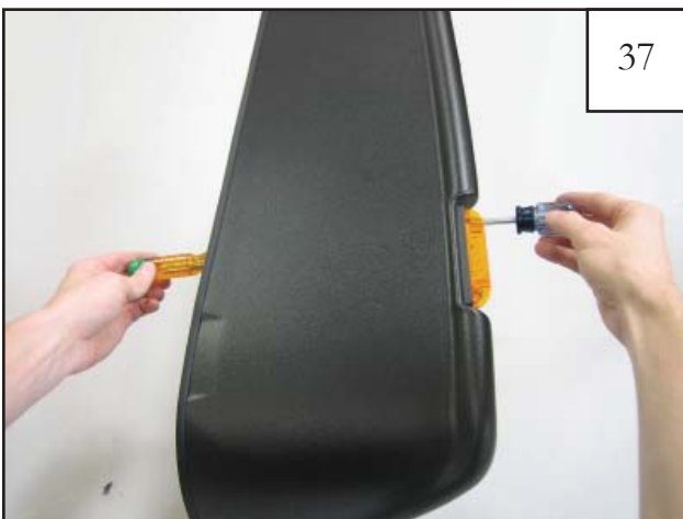
Secure the side marker light to the outer flare with 8-32 screw, 8-32 nut, and washer using a #2 Phillips bit and a 11/32" socket with 8" extension (2 places). NOTE: If you are having trouble putting the washer and nut on the screw, use needle nose pliers.
