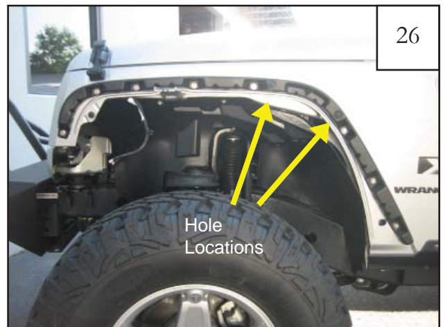
Secure inner pieces D7 (and P7 for passenger side installation) to the sheet metal using the following 2 Steps: Step 1 Position inner piece on fender, aligning with existing holes in first two inner pieces.
