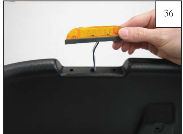
Position the supplied side marker light onto the outer flare piece, threading the wires through the center predrilled hole.
