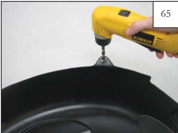
Use a drill and 5/16" drill bit to drill through mark made on rear mounting tab.
