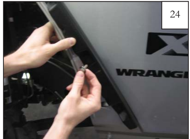
Step 2 Slide a .700" Washer onto 5/16" Hex Head Bolt. Insert a bolt/washer assembly through inner flare piece and fender and secure with 5/16" Nylok Nut. Start the bolts but do not tighten.
