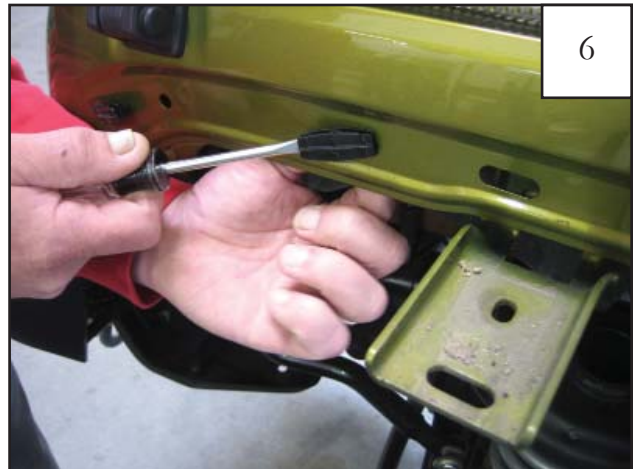
Using a pry tool or flat head screwdriver, remove any plastic clips still in fender.
