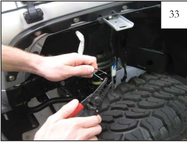
Use wire strippers to strip away approximately 3/8" of wire covering from the factory installed side marker lamp wires.
