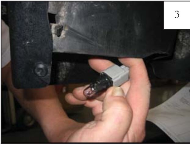
Remove light receptacle from light lens housing, letting it hang free of the housing.
