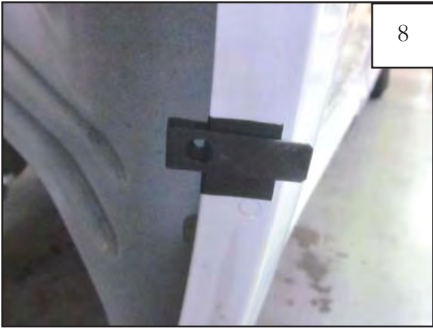
Install a Clip (CL1-0009) over each of the four Tabs (MT1-0034) placed over the upper 4 marks made in Step 16.
