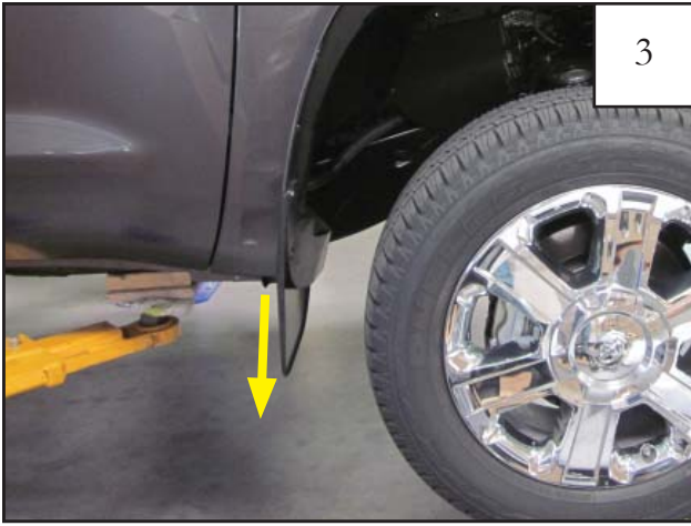
3 Remove push retainer from underside of factory mud guard.
