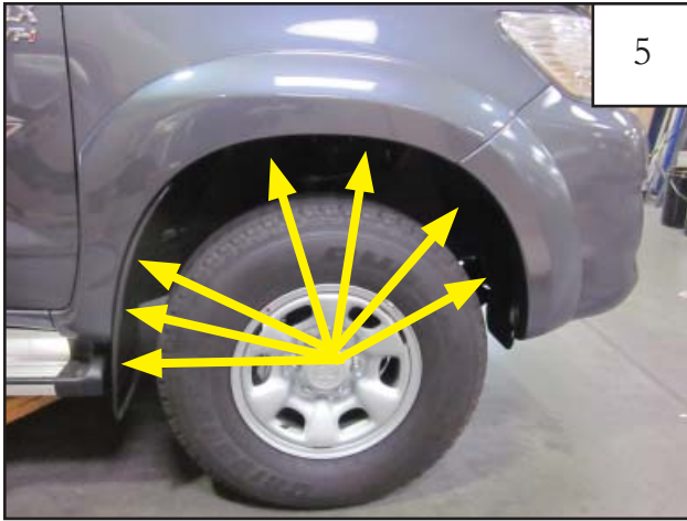
5 Remove seven factory screws from the fender lip. Save screws for reinstallation. Remove flare by pulling part away from side of vehicle.
