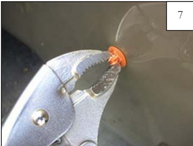
7 Remove two clips from front using vise grips, pulling with a rocking motion. See step 8.
