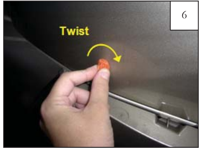
6 Using a clockwise twisting motion, remove six factory plastic clips from fender. See step 8.
