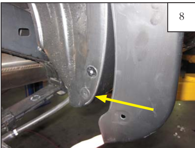
Remove factory installed grommet from lower front of the rear wheel well.
