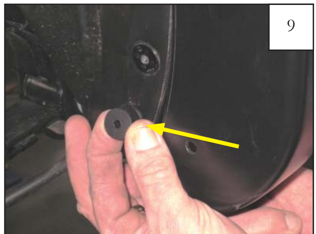
Install supplied grommet (GR1-0001) into factory hole.
