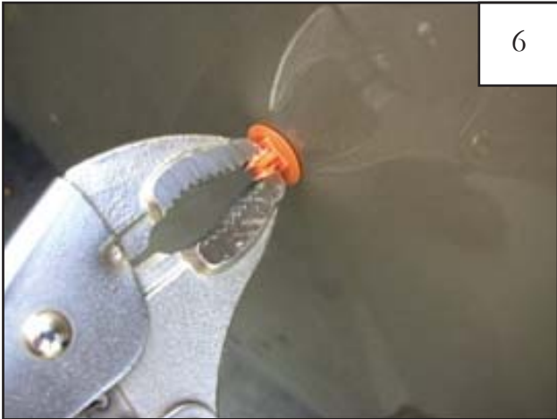
Remove one clip from fender using vise grips, pulling with a rocking motion. See Step 7.
