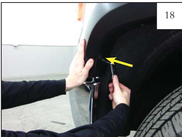
18 While holding Flare on vehicle, install factory screw removed in Step 7 through flare and into factory hole. Do not fully tighten at this time.
