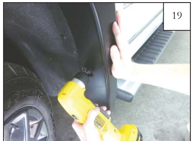
19 Install self-tapping screw (SW1-0066) into pilot hole drilled in step 16. Press flare towards vehicle while fully tightening. Note: This step not needed for models with factory installed mudflaps.
