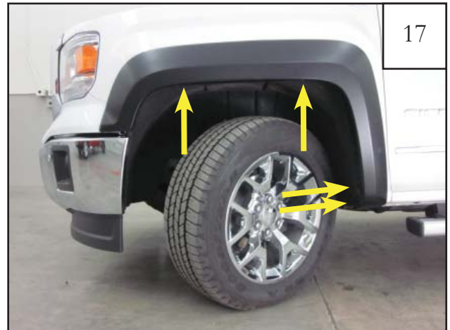
17 While holding Flare on vehicle, install supplied screws (SW1-0056) into the two upper and lower factory holes locations. Do not fully tighten at this time.
