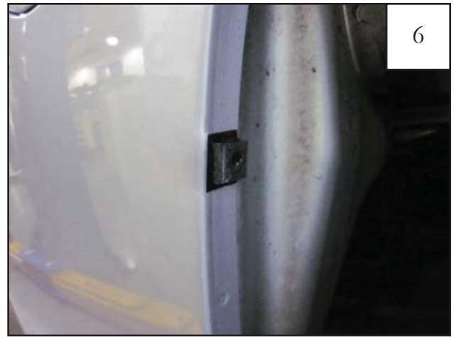
Slide a supplied Clip (CL1-0005) over each Tab at remaining four locations. Clips may need to be adjusted to align with holes in flare.
