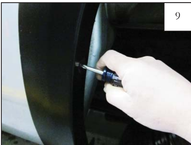
Start a supplied Screw (SW1-0050) through each of the remaining holes and into each Clip installed in Step 6. If needed, use scratch awl to locate holes.
