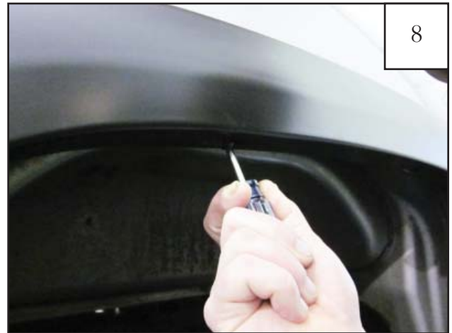
Reposition flare on fender, Start a supplied Screw (SW1-0058) through the two uppermost holes in the flare and into each Clip installed in Step 4.
