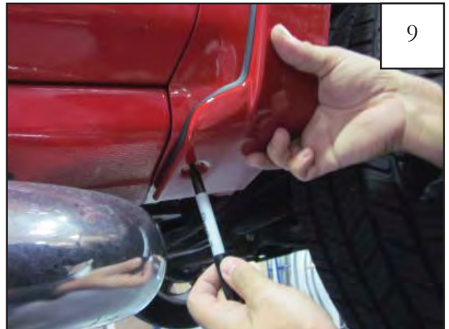
While still holding front of the flare firmly on the fender. Make sure front of flare is aligned with bumper style line. Using a grease pencil, mark the bottom fastener location using flare as guide.
