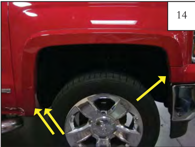
Locate flare into position on vehicle. Install supplied screw (SW1-0056) through two bottom rear holes in flare and into factory hole in front of wheel well.
