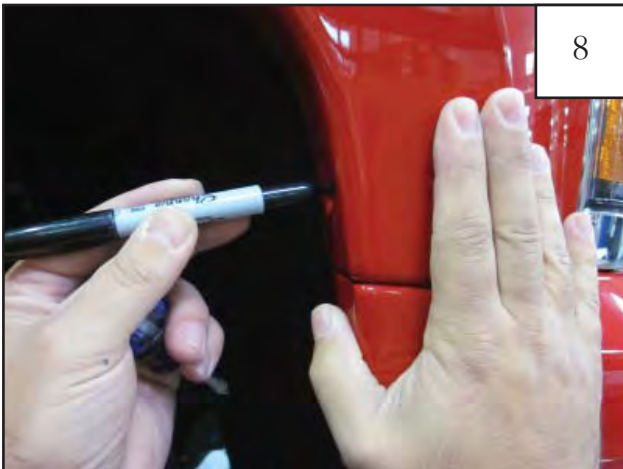
Hold front of the flare firmly on the fender. Make sure front of flare is aligned with bumper style line. Using a grease pencil, mark five hole locations using the holes in the flare as a guide. See next step.
