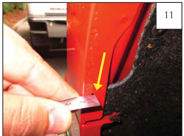
Remove the flare. At the marked location made in Step 8, measure inward 10mm from the edge of the fender. These are the marks to be drilled. Note: Marks at 10mm may be on either side of the first mark.
