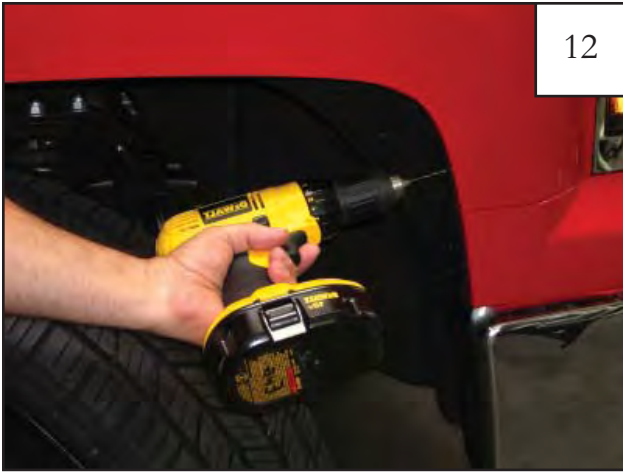
Using a 3/32" drill bit, drill pilot holes at the marks made in Step 11.
