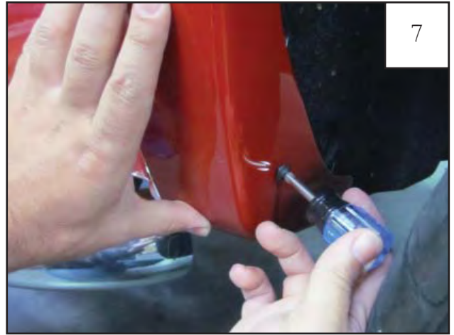
Place flare on vehicle and start supplied Screw (SW1-0056) through two bottom rear holes in flare and into factory hole in front of wheel well. Do not tighten.
