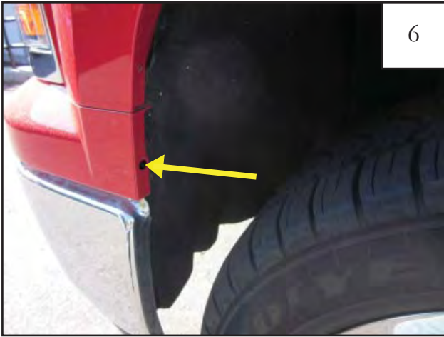
FOR 1500 MODELS ONLY: Using a 7mm socket, remove factory screw at bottom front of wheel well.
