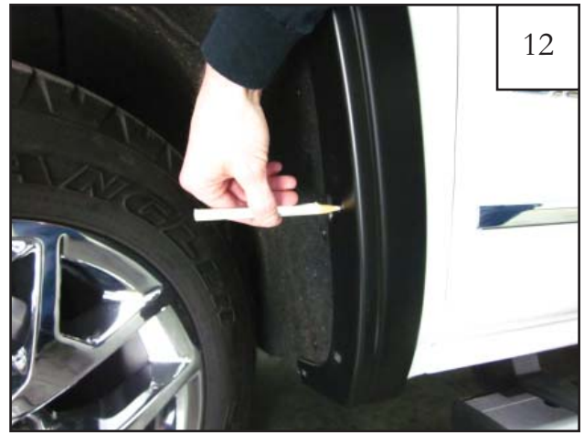
12 Using a grease pencil or marker, mark one hole location for drilling using the upper rear hole location in the flare as a guide. Note: This step not needed for models with factory installed mudflaps.
