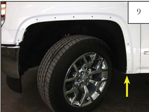
Reinstall factory fastener removed in step 9 using a 1/2" socket and wrench.
