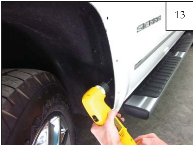
13 Remove the flare. Using a 3/32" drill bit, drill a pilot hole through the factory wheel well liner and sheet metal at location marked in previous step.
