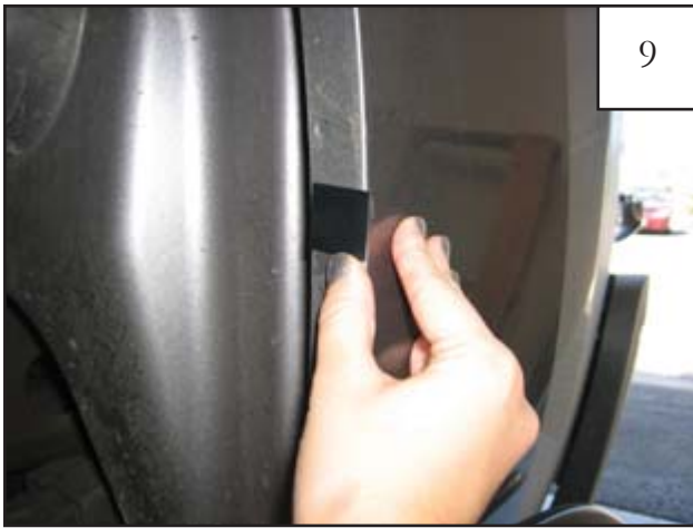
Center a supplied Tab (MT1-0002) over the marks made in step 7, aligning edge of tab with inside edge of fender lip (tab may extend over outside of fender).
