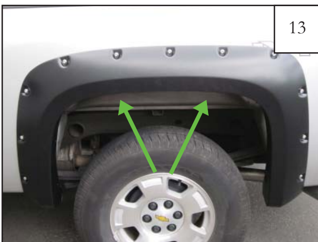
Reposition flare on fender. Start a supplied Screw (SW1-0058) through upper two hole locations and through each Clip (CL1-0022) installed in step 11. If needed, use awl to locate holes thru tabs installed in step 10.
