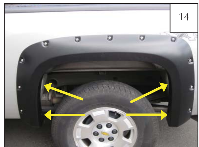
Start a supplied Screw (SW1-0050) through each of the remaining holes and into each Clip (CL1-0005) installed in step 12. If needed use awl to slide clips to meet hole locations in flare.
