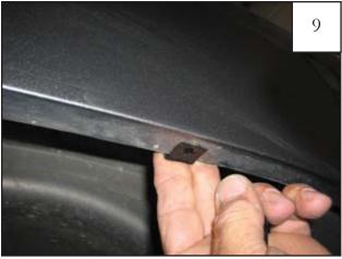
Center a supplied Clip (NU1-0007) over the upper two marks made in Step 7. Clips may need to be adjusted to align with holes in flare. *Note: The raised* collar on the Clip should face upward into the interior of the fender.
