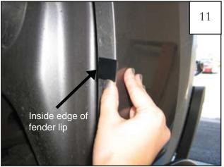
Center a supplied Tab (MT1-0002) over the six remaining marks made in Step 7, aligning edge of Tab with inside edge of fender lip (Tab may extend over outside of fender).
