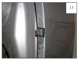
Slide a supplied Clip (CL1-0005) over each Tab. Clips may need to be adjusted to align with holes in flare.
