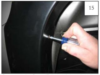
Start a supplied Screw (SW1-0050) through each of the remaining holes and into each Clip installed in Step 13. If needed, use scratch awl to locate holes.
