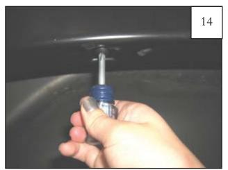
Reposition flare on fender, Start a supplied Screw (SW1-0057) through the two uppermost holes in the flare and into each Clip installed in Step 9.
