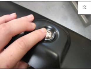
Put each Bolt through a pocket hole in the flare, bolt head on the outside.
