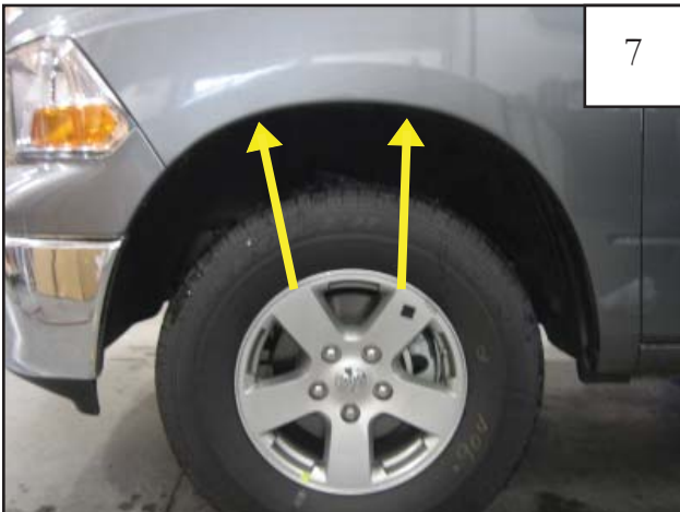
Install #10 U-Clips (CL1-0022) at these locations. See step 9. NOTE: There are two factory holes near the rearward arrow. The correct hole for install is the one more toward the front of the vehicle.
