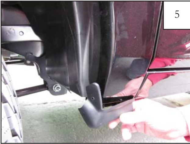
2011-up Models Only (Optional): If you encounter a fit problem, remove inner piece at bottom of front and rear wheel well.
