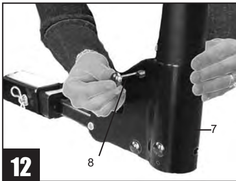
12 Insert 2.5" Carriage Bolt (short one) into square hole in tilt bracket.
