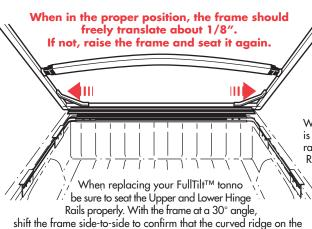
lower hinge rail is located between the tonno frame corner caps.
