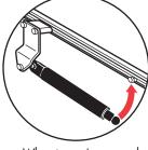
When tonno is removed, stow the gas shock against the shock hold down stud.
