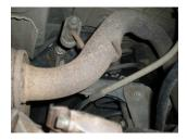
Using a hacksaw or sawsall, cut the stock tailpipe off where it exits the muffler. (This step is not mandatory, but it makes removal a little easier.)
