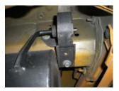
7) Install the OEM hanger bracket removed from the rear of the factory muffler onto the rear hanger of muffler #852467-231. Place the muffler up into position and connect the muffler inlet to the over-axle pipe. Bolt the hanger bracket to the frame using the OEM hardware from Step 2.
