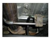
3) Place inlet pipe **#26354S** into position behind the front flange and connect the hanger on the pipe to the rubber mount on the vehicle. Then connect the two flanges together and use the supplied 3/8" bolts, nuts and washers to secure the two together. Be sure to square up the two flanges to each other and tighten enough to hold but still allow for adjustment.
