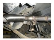
7) Place a provided 2½" clamp onto the slip-fit of the left tailpipe rear section **#16716S**. Then place the slip-fit over the back of the front section and connect the hanger at the rear of the pipe to the rubber mount on the vehicle. Tighten the clamp on the slip connection enough to hold but still allow for adjustment.
