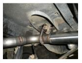
5) Place a provided 2½" clamp onto the right muffler outlet. Place tailpipe **#16715S** into position over the rear axle and into the right muffler outlet. Connect the hanger at the rear of the tailpipe to the rubber mount on the vehicle. Tighten the clamp on the outlet enough to hold but still allow for adjustment.
