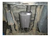
4) Place the provided 3" clamp onto the muffler inlet then slide onto the back of the inlet pipe. Support the muffler with a stand and tighten the clamp enough to hold but still allow for adjustment.
