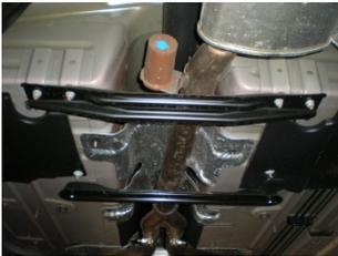
1) Raise the vehicle and support securely with stands. To ease the removal of the stock system, spray a penetrating lubricant onto all of the rubber hangers of the system. Use a 13mm socket to loosen the six nuts attaching the two factory body braces to the underside of the vehicle, set the braces aside for re-installation in step 4 below.
