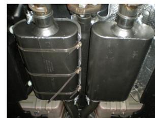
5) Place a supplied 2 1/2" clamp onto the inlet of each muffler **#842551-Z**. Then fully slide the mufflers onto the back of the Scavenger pipe assembly and support with stands. Level the mufflers and tighten the clamps enough to hold, but still allow for adjustment.
