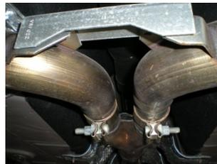
3) Support the right side muffler with a stand, then using a 15mm socket, loosen the clamps at the Y-pipe connection behind the catalytic converters. Remove the four remaining hanger rods from the rubber mounts on the vehicle and slide the system back off of the head pipes.
