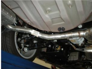
2) Use a 15mm socket to loosen the clamp at the slip-fit connection just forward of the left muffler behind the Y-pipe. Slide the two hanger rods out of the rubber mounts on the vehicle and remove the left muffler assembly.
