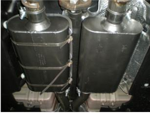
6) Because the factory exhaust system has only one muffler, there is no heat shielding on the left side of the vehicle. To provide heat shielding to the left muffler, place the **#51017** heat shield onto the top of the left muffler and secure with the stainless hose clamps provided in the kit.
