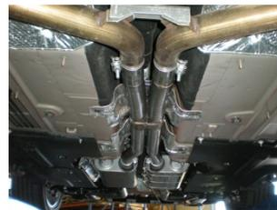
4) Begin by placing a supplied 2 1/4" clamp onto each of the slip-fits of Scavenger pipe **#16705S**. Then place the Scavenger pipe onto the back of the stock head pipes (make sure the Flowmaster embossing is facing the ground). Level and center the assembly in the drive line tunnel and support with a stand. Tighten the two clamps enough to hold, but still allow for adjustment. Reinstall the two factory body braces removed in Step 1 above and tighten securely.
