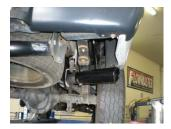
8) Place the **ST396** stainless tip onto the end of the tailpipe and adjust to the desired location. Tighten the nut on the clamp to secure the tip in place.
