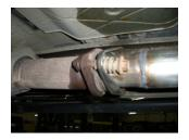
5) Using the factory bolts, springs and flag nuts, connect the flange on inlet pipe **#16707S** to the flange behind the catalytic converter. Tighten securely.
