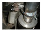
6) Place a 2½" band clamp onto the inlet of the muffler and place onto the rear of inlet pipe **#16707S**, support the muffler with a stand. Tighten the clamp enough to hold but still allow for adjustment.
