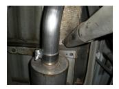
7) Place a provided 2½" clamp onto the muffler outlet. From the rear of the axle, place the tailpipe **#16708S** over the axle and into the muffler outlet. Connect the wire hanger at the rear of the pipe to the rubber mount on the frame. Tighten the clamp enough to hold but still allow for adjustment.
