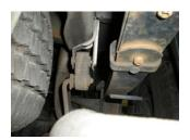
1) Raise the vehicle up to working height and support securely. Begin by spraying a penetrating lubricant onto the front flange bolts as well as the rubber hangers that support the factory exhaust system. Then, using a hacksaw or sawzall, cut the tailpipe just behind the muffler. Remove the hanger at the rear of the tailpipe from the rubber mount on the vehicle and lower the tailpipe from the vehicle.
