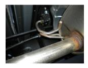
2) Use a hacksaw or sawsall to cut the stock tailpipe off where it exits the muffler. This step is not required but makes removal of the stock system much easier. Once cut, slide the tailpipe toward the front of the truck to remove the hanger at the rear of the tailpipe from the rubber mount on the vehicle.
