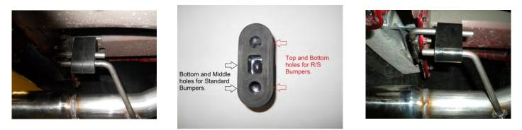
11) Place a provided clamp over the left Y-pipe outlet. Slide the expanded end of the left tailpipe **#16752S** onto the Y-pipe outlet and connect the hanger at the rear of the pipe to the rubber mount installed in step 10 above. Tighten the clamp enough to hold, but still allow for adjustment.
