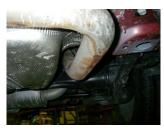
3) Your second cut will be just before the pipe goes up over the rear axle; this will allow the rest of the system to be removed easily. After cutting, support the rear muffler with a stand and remove the two hangers on this section from their rubber mounts. You can now lower this rear section from the vehicle.
