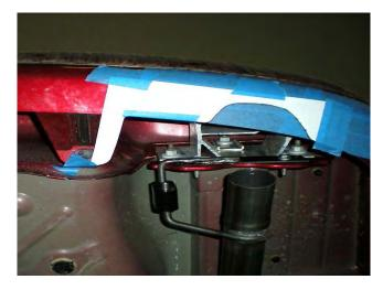
2) Use scissors to carefully cut out one of the provided paper templates and securely tape it to the bumper. Make sure to follow the lines on the body as well as the bumper mount to line up the template properly. *There are two templates included, one for the R/S package bumper and one for the standard models.*
