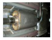
6) Place a supplied clamp onto the muffler inlet and slide onto the back of the inlet pipe. Level the muffler and support with a stand. Tighten the clamp just enough to hold, but still allow for adjustment.
