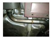
7) Place a supplied clamp onto the muffler outlet, then slide the short end of mid pipe **#16746S** into the muffler outlet and support with a stand. Tighten the clamp at the muffler outlet enough to hold, but still allow for adjustment.
