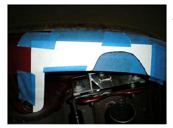
3) Use a marker and trace the cut-out template onto the masking tape. Remove the template after marking.
