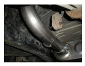
6) Place a supplied clamp onto the muffler outlet then place pipe **#86024S** into position and connect the hanger on the pipe to the rubber mount on the vehicle. Once the hanger is connected, place the pipe into the muffler outlet. Tighten the clamp enough to hold, but still allow for adjustment.
