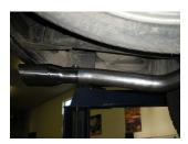
8) Place the **#ST446** stainless tip onto the end of the exit pipe and adjust to the desired position. Tighten the clamp on the tip enough to hold, but still allow for adjustment.
