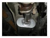
5) Place a supplied clamp onto the muffler inlet, place the muffler onto the back of the inlet pipe, the muffler outlet will be toward the outside of the vehicle. Support the muffler with a stand and tighten the clamp enough to hold, but still allow for adjustment.
