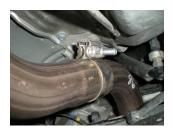
5) Place a provided clamp onto the expanded end of intermediate pipe **#16776S** and slide onto the back of inlet pipe **#16775S**. Rotate the pipe up into its approximate position and tighten the clamp enough to hold but still allow for adjustment. **For 2 door model vehicles:** 2.00" must be trimmed from the back of intermediate pipe #16776S prior to installation.
