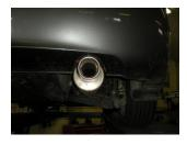
8) Place the **ST402** stainless tip onto the muffler outlet and adjust to the desired position. Tighten the clamp enough to hold, but still allow for adjustment.
