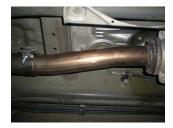
4) Place inlet pipe **#16783S** onto the back of the catalytic converter and rotate so that it is centered in the center channel of the vehicle. Replace the three nuts removed in the previous step and tighten securely. **Note: For 2 door model vehicles, trim 2.00" from the back of inlet pipe #16783S.**
