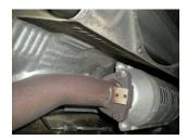
3) At the center of the vehicle, remove the three nuts at the flanged connection behind the catalytic converter. Once the flange is loose, remove the three hangers at the rear of the assembly from the rubber mounts on the vehicle and lower the front pipe/resonator from the vehicle.
