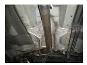
5) Place a provided clamp onto the front of resonator assembly **#15164S** and slide onto the back of the inlet pipe **#16783S**. Rotate the assembly up into its approximate position and connect the hanger on the pipe to the rubber mount on the vehicle. Tighten the clamp enough to hold but still allow for adjustment.
