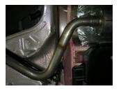
5) Place a supplied 2¼" clamp onto the muffler outlet, then slide the short end of mid pipe **#16820S** into the muffler outlet and support with a stand. Tighten the clamp at the muffler outlet enough to hold, but still allow for adjustment.
