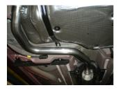
5) Place a supplied 2½" clamp onto the resonator outlet, then slide the front end of mid pipe **#16837S** into the resonator outlet and support with a stand. Tighten the clamp at the resonator outlet enough to hold, but still allow for adjustment.
