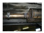
5) Place one of the provided 2½" clamps onto the muffler inlet and then slide the muffler onto the inlet pipe and support with a stand. Tighten the clamp enough to hold but still allow for adjustment. The outlet of the muffler will be toward the outside of the vehicle.
