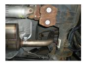
6) Place a provided 2½" clamp onto the muffler outlet and then place tailpipe **#16811S** into position over the axle. Insert the hanger at the rear of the tailpipe into its rubber mount on the vehicle and then slide the front of the pipe into the muffler outlet. Connect the front hanger to the rubber mount on the vehicle and tighten the clamp enough to hold, but still allow adjustment.
