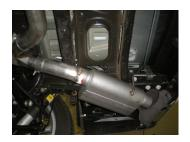
Place a provided 3" clamp onto the inlet of the right resonator assembly #15169S. Place the assembly up into position and connect the hanger on the assembly to the rubber mount on the vehicle. Slide the assembly to the rear and then slide the inlet onto the right y-pipe outlet. Slide the pipes fully together and tighten the clamp at the inlet enough to hold, but still allow for adjustment.
