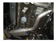
7) Place a provided 3" clamp onto the inlet of the left resonator assembly #15170S. Place the assembly up into position and connect the hanger on the assembly to the rubber mount on the vehicle. Slide the assembly to the rear and then slide the inlet onto the left y-pipe outlet. Slide the pipes fully together and tighten the clamp at the inlet enough to hold, but still allow for adjustment.
