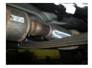
3) Support the large muffler in the center of the vehicle with a stand and remove the hangers on the muffler and over-axle pipe assembly from the rubber mounts on the vehicle. Loosen the clamp at the ball connection behind the catalytic converter and with the help of an assistant, lower the remainder of the system from the vehicle. The clamp will be re-used with the Flowmaster system.
