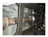
4) Place inlet pipe **#599TBS** into position behind the catalytic converter and connect the hanger on the pipe to the rubber mount on the vehicle. Then using the factory clamp secure the inlet pipe to the converter. Be sure that the hanger is level and tighten the clamp enough to hold, but still allow for adjustment. Place the provided 4" clamp over the back of the inlet pipe in preparation for the next step.
