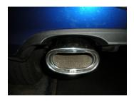
8) Place stainless **#ST465** onto the back of the over-axle pipe and adjust to the desired position. Tighten the clamp on the tip enough to hold, but still allow for adjustment.
