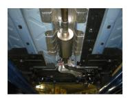
5) Place a provided 2" clamp onto the muffler inlet and slide onto the back of inlet pipe **#16876**. Tighten the clamp on the muffler inlet enough to hold, but still allow for adjustment.
