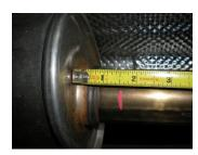
3) The system will now need to be cut just in front of the mid resonator assembly. Measure forward 1.50" from the end cap of the resonator and make a mark, support the resonator with a stand. Then using a hack saw or sawzall, cut through the pipe on your mark. Remove the hanger on this section from the rubber mount on the vehicle. Lower the resonator and over-axle pipe from the vehicle.
