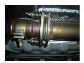
5) Take the provided M10-1.5x60mm bolts and slide on the flat washer. Then, put the bolts through the flanges and slide on the provided steel spacer sleeves and the springs and nuts removed in step 2 above. Tighten down the fasteners until the nuts bottom out on the steel spacer sleeves.
