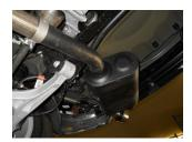
6) Place a provided clamp onto the inlet of muffler **#852559-300** and put up into position onto the outlet of the Y-pipe assembly. Slide the pipes fully together and connect the two hangers on the muffler assembly to the rubber mounts on the vehicle. Tighten the clamp at the inlet enough to hold, but still allow for adjustment.
