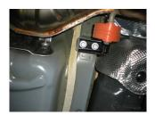
3) After the system has been lowered from the vehicle, remove the two bolts that attach the first set of factory hangers behind the front flange connections. Retain the bolts; these hangers will be replaced with the **#453HA** hangers included in the parts kit.
