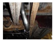
4) Take the **86076S** muffler inlet pipes and place a supplied 2½" clamp onto the expanded end, place them onto the back of the H-pipe assembly's **86074S** & **86075S**. Rotate them up into their approximate position and tighten the clamps enough to hold, but still allow for adjustment.
