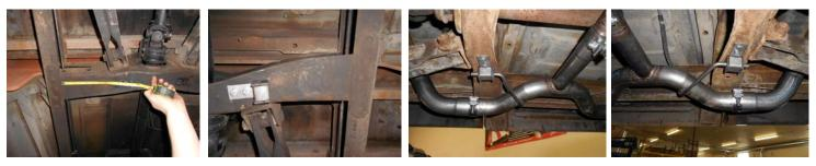
2) Take the right and left H-pipe assemblies, **86074S** & **86075S** and connect them together at the center cross-over connection. Place them up into position and connect the hangers on the pipe to the rubber mounts installed above. The hanger rods should stick through the rubber block on the **HA572** hanger approximately 1.00". Support the front of the assembly with a stand. Place the provided 2" clamp at the center H-pipe connection.
