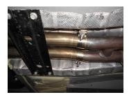
5) Install a provided 2 ¼" clamp onto the reduced and Z-notched end of intermediate pipe #86207\$. Slide the pipe onto the right factory front pipe as far as it will go and rotate to its approx. position in the drive line tunnel. Support the rear of the pipe with a stand and tighten the clamp enough to hold, but still allow for adjustment. Repeat this step with pipe #86208\$ on the left side of the vehicle. You can now reinstall the black body brace, tighten securely.
