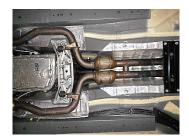
4) Reinstall the front (rear converter) portion of the system by reconnecting the two hangers on the assembly to the rubber mounts on the vehicle and reinstalling the two bolts on each of the two flanged connections behind the front converters. Tighten securely.
