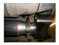
2) Place the left side stainless tip **#ST434** over the left muffler outlet, the **484HA** clamp hanger with fit over the tip. Adjust the tip to the correct position and tighten the clamp enough to hold, but still allow for adjustment. Repeat this step with tip **#ST433** on the right side of the vehicle.
