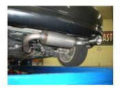
6) Place a provided 2.50" clamp onto the inlet of muffler #12514310-Z and slide onto inlet pipe #16689S. Support the muffler with a stand and tighten the clamp enough to hold the muffler in position, but still allow for adjustment.
