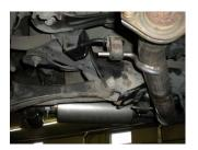
5) Place inlet pipe **#16689S** into position behind the factory flange and connect the two hangers on the pipe to the rubber mounts on the vehicle. Then using the two M10x1.25 hex nuts provided, re-install the two bolts removed in step 2 above and tighten securely.
