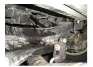
4) Using the 3/8" bolt, nut and washers provided in the parts kit, bolt hanger #420HA to the rear axle in the hole indicated by the photo at left. Tighten securely. Then place the provided #HA168 rubber hanger onto the round stock portion of hanger of #420HA.
