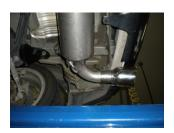
7) Place a provided 2.50" clamp onto the outlet of the muffler, then place exit pipe **#16690S** into the outlet and connect the hanger on the pipe to the rubber mount on the vehicle. Tighten the clamp enough to hold, but still allow for adjustment.
