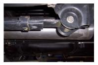
INSTALL MUFFLER #B ONTO HEAD PIPE 1-1/2" TO 2" WITH THE LOUVERS FACING TOWARDS THE CONVERTER. THE MUFFLER OUTLET SHOULD BE POSISTIONEDTHE MUFFLER OUTLET SHOULD BE POSITIONED AT 12:00. USE A JACK STAND TO SUPPORT THE MUFFLER. USE CLAMP #E TO SECURE THE MUFFLER TO THE HEAD PIPE. DO NOT TIGHTEN. MUFFLER INLET IS LOOKING INTO THE LOUVERS.
