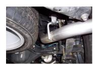
INSTALL THE OVERAXELE TAILPIPE #C INTO THE MUFFLER 1-1/2" TO 2". DO NOT TIGHTEN.
