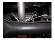
5. Slide the over axle tailpipe #C into the muffler 11/2"-2". Insert welded hangers into rubber grommets. Use clamp #E to secure the muffler and tailpipe together. Do not tighten.
