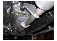
3. Install headpipe #A at the 2-bolt flange connection. Secure with bolt kit #F. Do not tighten. Insert welded hanger into rubber grommet.
