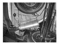
INSTALL MUFFLER ASSEMBLY #C. SLIP THE WELDED HANGER INTO THE FACTORY RUBBER GROMMETS. RE-CONNECT THE GROUND STRAP TO THE MUFFLER ASSEMBLY USING BOLT KIT #F.
