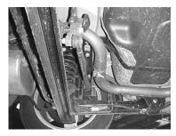
LAY OUT THE GIBSON EXHAUST AND COMPARE PARTS TO THE MANUAL. DISCONNECT THE GROUND STRAP CONNECTED TO THE FACTORY PIPE BEHIND THE MUFFLER. DISCONNECT THE FACTORY MUFFLER IN FRONT OF THE AXLE. THEN REMOVE THE MUFFLER. LEAVE ALL FACTORY RUBBER GROMMETS IN PLACE.
