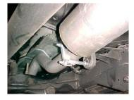
Install muffler onto head pipe 1-1/2" to 2" with the louvers facing towards the converter. Use a jack stand to support the muffler. Use front muffler hanger # E to secure muffler to headpipe. Insert hanger into rubber grommet. Do not tighten. Muffler inlet is looking into the louvers.
