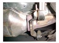
Lay out the exhaust on the floor so it looks like the drawing and compare parts with manual. Remove your stock exhaust from the 2-bolt flange located just behind the catalitic converter. You will re-use you factory gasket & hardware. Leave all rubber grommets in place. Use WD-40 to aid in removal of exhaust and hangers.
