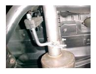
Use rear muffler hanger # F to secure tailpipe to muffler. Insert hanger into rubber grommet. DO NOT TIGHTEN.
