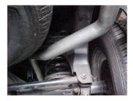
Install the over axle tailpipe # C into the muffler 1-1/2" to 2" and insert welded hanger into rubber grommet.
