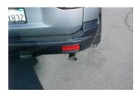
Install stainless steel tip. Clamp down. When you have everything in place, firmly tighten all bolts and clamp down securely. To clean stainless steel tip use any stainless steel cleaner and Scotch Brite pad.
