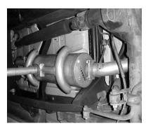
SLIDE MUFFLER WITH DUAL INLET ONTO HEADPIPE AT LEAST 1-1/2" TO 2". MUFFLER OUTLET SHOULD BE AT THE 5 O'CLOCK POSITION. USE CLAMPS #F TO ATTACH TO THE HEADPIPE. MAKE SURE INLETS AND THE MUFFLER IS LEVEL. AND TIGHTEN DOWN. USE JACK STAND TO SUPPORT MUFFLER.
