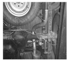
INSTALL THE OVERAXLE TAILPIPE #C INTO MUFFLER AT LEAST 1 1/2" TO 2" USING CLAMP #G. DO NOT TIGHTEN. INSERT WELDED HANGERS INTO RUBBER GROMMETS. THE SPARE TIRE ON SOME VEHICLES MAY NEED TO BE LOOSEN ED AND PULLED TO THE DRIVER SIDE AND RE-TIGHTENED. **ROTATE PIPES UNTIL YOU** HAVE AT LEAST A 1" **CLEARANCE AWAY FROM** ALL PIPES, ETC.
