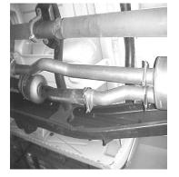
INSTALL DRIVERSIDE HEADPIPE #A AND PASSENGER SIDE HEADPIPE #B WITH O2 SENSOR, OVER THE FACTORY HEADPIPES NO LESS THAN 1 ½" AND NO MORE THAN 2". INSERT WELDED HANGER INTO RUBBER GROMMET. USE CLAMPS #I TO CLAMP DOWN HEADPIPES.
