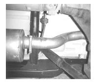
INSTALL MUFFLER #C WITH THE OUTLET LOCATED AT 12:00 O'CLOCK. ATTACH CLAMP #G AT THE MUFFLER INLETS (DO NOT TIGHTEN). USE A JACKSTAND TO SUPPORT MUFFLER. INSERT WELDED HANGER INTO RUBBER GROMMET.
