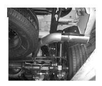
USE CLAMP #E TO SECURE THE PIPE TO THE MUFFLER. DO NOT TIGHTEN. INSERT WELDED HANGERS INTO RUBBER GROMMETS.
