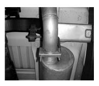
INSTALL MUFFLER WITH THE INSIDE LOUVERS FACING FORWARD TOWARDS THE CONVERTER. USE CLAMP #E AT THE INLET OF THE MUFFLER. DO NOT TIGHTEN. MUFFLER OUTLET WILL BE POSITIONED AT ABOUT 11 O'CLOCK. THE MUFFLER INLET IS LOOKING INTO THE LOUVERS.
