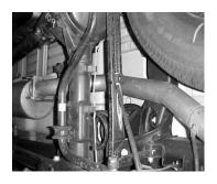
INSTALLTHE OVER AXLE TAILPIPE #C INTO THE OUTLET OF THE MUFFLER 1  $\frac{1}{2}$ " TO 2". DO NOT TIGHTEN.
