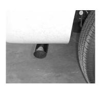
INSTALL THE STAINLESS STEEL TIP. USE ANY ALUMINUM OR STAINLESS CLEANER TO POLISH YOUR TIP.NOW, FIRMLY TIGHTEN ALL CLAMPS, HANGERS AND FLANGE.
