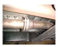
Lay out the exhaust on the floor so it looks like the drawing and compare parts with manual. To remove your stock exhaust Remove it from the 2-bolt flange located in front of the muffler. Then cut off your tailpipe. Leave all rubber grommets in place. Use WD-40 to aid in removal of exhaust and hangers.
