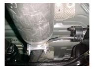
Next install front muffler hanger #E onto muffler. Insert hanger into rubber grommets. Do not tighten.
